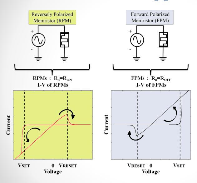
Memristors with opposite polarities present reversed behavior (flipped *I–V* characteristic)
